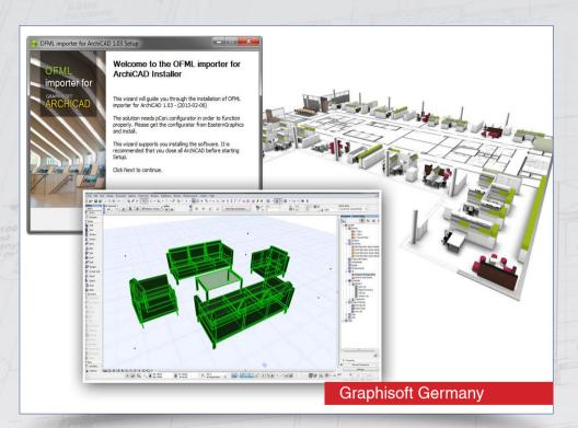
This tool was created for Graphisoft Germany. OFML based objects can be imported into ArchiCAD 16 via pCon. configurator from Eastern Graphics. The solution makes sure that the products of German furniture manufacturers can be placed and used in ArchiCAD 16.
