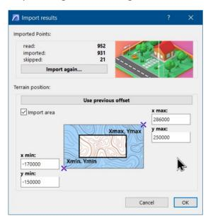
When this option is activated, it allows to import an area which the user can define, through the four activated fields (Xmin, Ymin, Xmax and Ymax).
