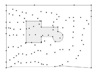
To create a plateau, first draw the perimeter of the area to be levelled using the fill tool and then select the fill to be processed.
