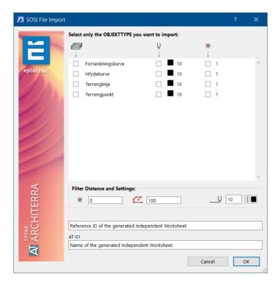
By selecting the layers, filter distance and settings, the import results dialog box with the number of imported data will open.
