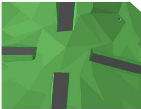
Before created a junction, make all the necessary modifications to the altitudes of the road levels until obtain the desired situation (thus avoiding the need to manually reconfigure the altitudes of the junction nodes during subsequent phases).
