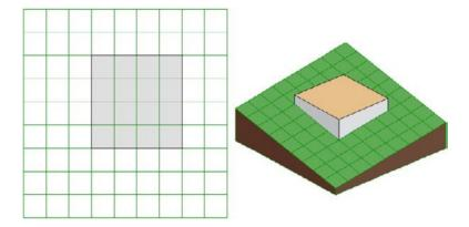
The above image shows a simple Mesh constructed with ARCHICAD into which a Slab has been inserted.
