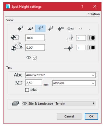
In the View section, it can be configured the appearance of the marker by choosing the style and defining the dimensions, angle and pen used to draw it. In the Text section, it can be chosen the font, size of character and possible use of italics for the string of information to be displayed.
