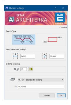
The drawing option using the two buttons on the dialog box can be chosen to define the type of outline: polygon or rectangle.
