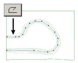
Next, select the ARCHICAD polyline defining the route where the cameras will be distributed and finally click on the Camera tool icon in the ArchiTerraPlus toolbox.
