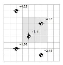
As can be seen in the image, ARCHICAD still attributes spot heights at the original surface altitude (prior to the Boolean subtraction operations) without considering the modifications made using Solid Elements Operations.
