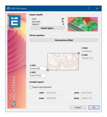
In this case, the user can use the same coordinates as used for the worksheet before (if it was created one) or choose new values. The user can also add and altitude filter for their imported data, considering the first altitude and the final, besides the equidistance between the points.
