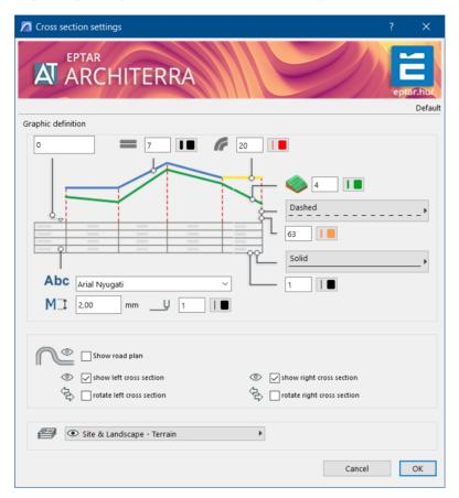
The numerical field at the top left enables to set the reference altitudes (within the limits of the interval available). The user can use this field, for example, to align the various longitudinal sections and make them congruent.
