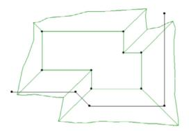
Select the element to be limited (in our example, a plateau) and the polyline representing the obstacle and then click on the Retaining Wall icon in the ArchiTerraPlus toolbox.
