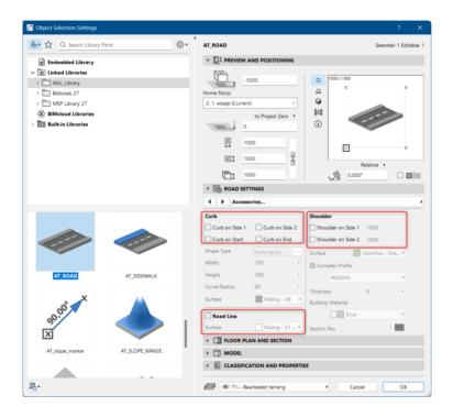
The road line and the curb is visible in 2D and 3D.
