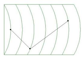
As explained above, when this polyline is transformed into an ArchiTerraPlus wall, ArchiTerraPlus will use the three nodes to acquire information on the altitudes of the terrain and then construct the resulting wall. Then select the polyline and the terrain/mesh and click on the Wall tool in the ArchiTerraPlus toolbox to display the Wall settings dialog box, confirming the default configuration.
