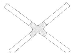
The junction, represented by a fill with 45° hatching, also contains curved parts. As explained in previous paragraphs, there are in fact no limitations to the shape.
