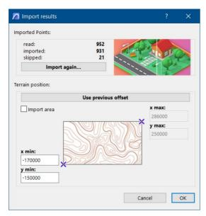
This can be resolved by using the two fields below in the Terrain position section to shift the data and reposition them near the origin: Delta X and Delta Y are the two values used to position the terrain.
