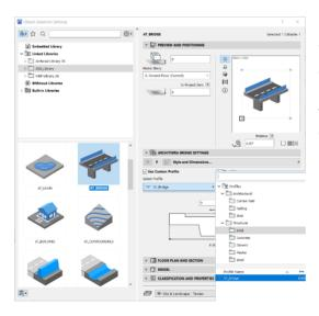
When you select a Custom profile the width of the bridge, the sidewalk and the pavement will the size what you defined in the Profile Manager. If you would like to change these sizes, you should edit the profile in the Profile Manager and save it.
