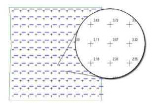
In this case, the entire map with spot heights is represented by a single AT3\_POINT\_MARKER object. To modify the characteristics, select the AT3\_POINT\_MARKER object and click on the Spot Heights tool icon, modify the parameters, and confirm with the OK button.
