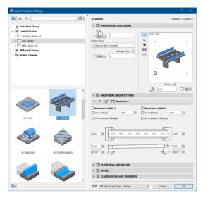
On the next TAB of the Bridge settings window, you are able to switch the Abutment on both ends of the Bridge. The size, the shape of the abutment (curved or rectangular), and the Inclined Angle of it can be set. You can also decide how the abutment connected to the deck of the bridge: fit to bottom of bridge or not.
