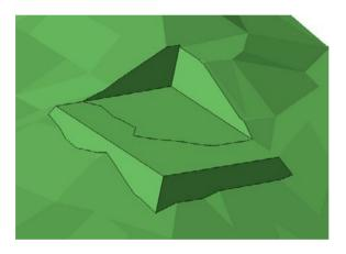
In a subsequent phase, the height of the plateau has been modified and raised appreciably. As can be seen from the following image, this graphic modification has left a block at the base where the original length of the scarp is no longer sufficient:
