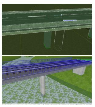
The position of the Piers is modifiable graphically with hotspots in 2D and 3D.
