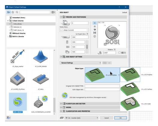
As a result, the terrain and different objects (buildings, roads, etc) will be converted from SOSI data into the 3D models.
