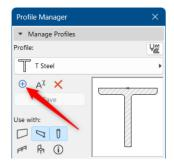
Open the profile manager, click on "+" sign. Give the name for this profile and save it into the existing or new folder in the profiles list.
