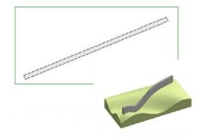
If you move the cursor to the two sides of the polyline, the arrow changes direction, indicating the side on which the Retaining Wall will be constructed. Click on the required side and ArchiTerraPlus immediately generates the element requested.
