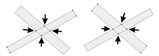
At the junction, each of the two roads will now have editable nodes that can be used to adjust their shape.
