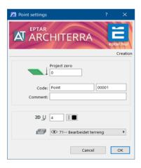
This starts the point insertion cycle and each time clicking on the worksheet, a new point with the characteristics defined in this box is inserted.
