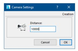
This dialog contains a single parameter the approximate distance between each camera along the route. Enter a value and confirm with the OK button.
