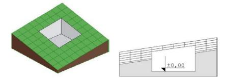
Using Solid Elements Operations, the volume of the slab is subtracted from the mesh: As can be seen in the cross section, the altitude of the mesh corresponding to the plateau obtained by subtracting the volume of the mesh is 0.00 meters.
