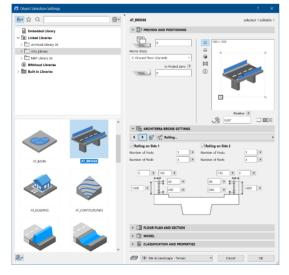
On the 4<sup>th</sup> tab of the Bridge settings the Railing can be set on both sides with size, position parameters. You can set the number of Posts and Rods separately, set the size of them.
