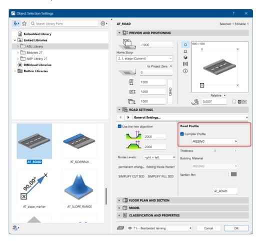
The composite, what could be used for road, is not predefined in Archicad, so it must be created in the Profile Manager by user.
