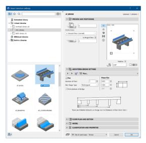
On the 3<sup>rd</sup> tab of the Bridge settings window, you can apply Piers, if the Bridge is too long. The size, the shape of the Pier (Rectangular, Curved rectangular, Oblong, and Circular), and the amount of them can be set. You can also decide how the pier connected to the deck of the bridge: fit to bottom of bridge or not.
