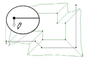
Once clicked the Retaining Wall icon, the procedure begins and the cursor changes to an arrow at the start of the polyline used to generate the obstacle.
