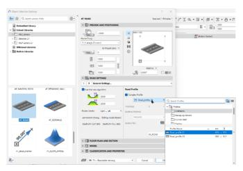
Now click on the Save button on the Profile Manager palette. The necessary composite is created and can be applied for Road.
