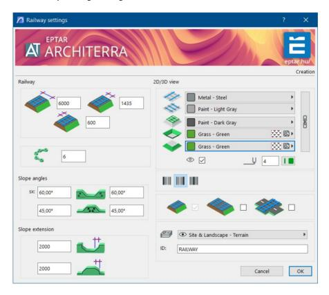
The first value in the Railway section indicates the width of the railway. Use a polyline to create Railway with a constant width.
