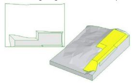
If the perimeter of the terrain is modified subsequently (in the following image, the hatched part of the map indicates the new perimeter of the terrain), for example by creating indentations, the result will be a "projecting" terrain as the shape of the original perimeter has been modified:
