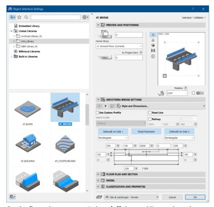
On the first tab you can switch on/off the road line and set the custom profile for the bridge deck, even for Railway bridge. The default profile is a simple slab, no in this case you can define the sidewalk on both side and the pavement.
