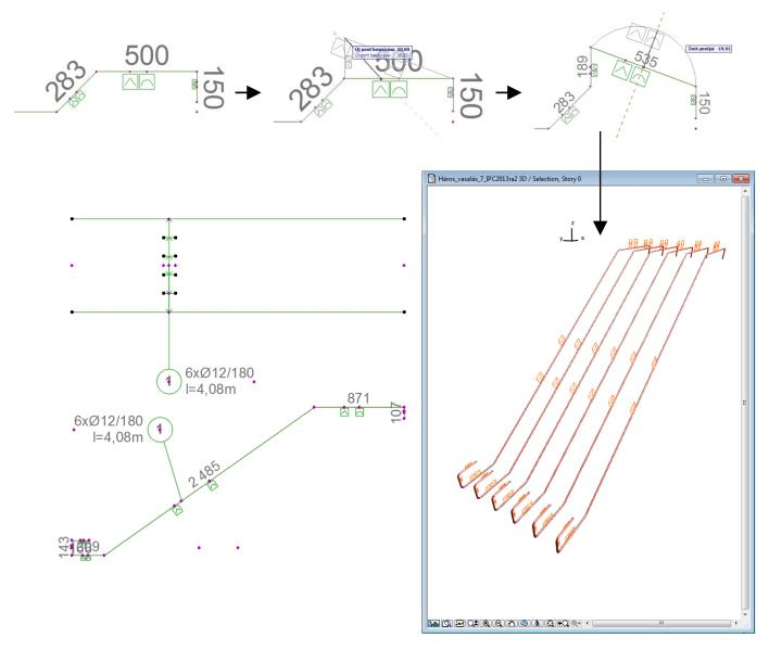
If you want to delete a corner from the polyline move it over the next corner point, the solution will remove the line sections of 0 cm length and the two corner points will be merged.
