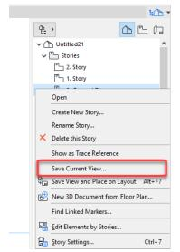
On the right side on "**Navigator**" palette under the "**Project Map**" tab, click right the name of the active layout. Choose "**Save Current View...**" command. Give the view an easy, typical name (e.g. "**Downstairs – Reinforcement plan**").
