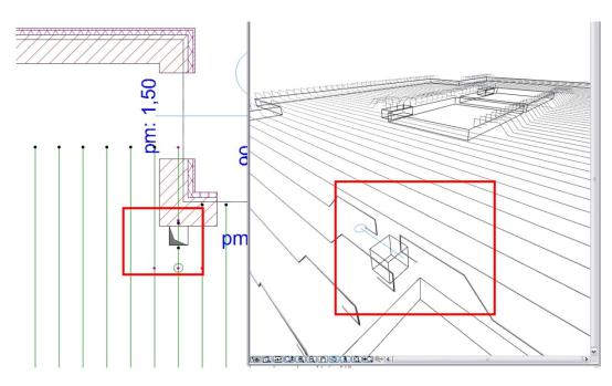
The rebars and meshes - which have been placed with Eptar Add-on – will be grouped together, so the styles of the rebar or meshes will be in one placed group.
