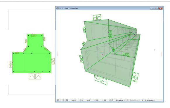
This objects are not available in the cutting list and do not count in the Rebar optimalization method.
