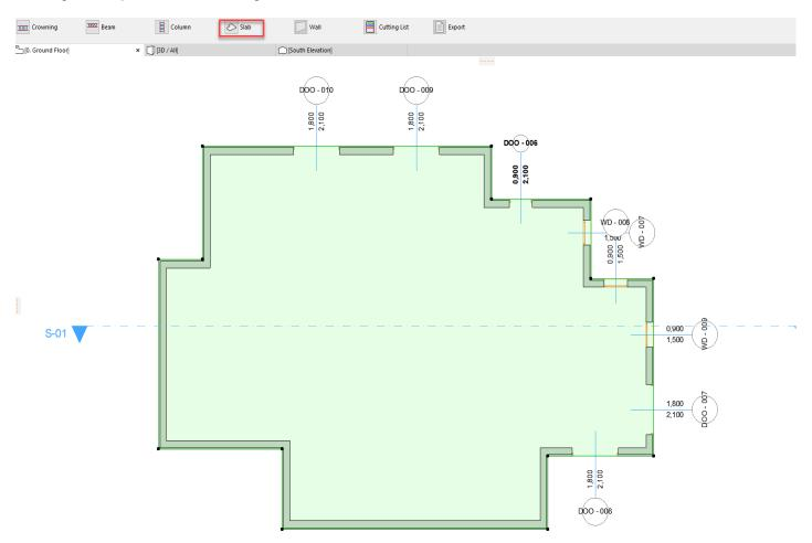
Select the ArchiCAD slab or wall objects to fill out with rebar or mesh elements. Use "**Floating palette / Slab or Wall**" command. Select the rebar or mesh object in the dialog box and set up the necessary parameters as we defined in the earlier chapter. Click "OK" button, the ArchiCAD automatically places the rebar or mesh elements into the polygon shape slab or wall with the parameters already defined.
