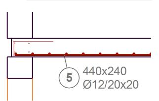
If you choose mesh objects, maybe the mesh section view will be shorter or longer as the original object section view. In this case, you can edit the length of the mesh's section view with the hotspots on the edges.
