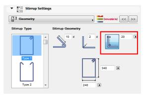
Select stirrup section form and set up the parameters on the "Geometry" tab page.
