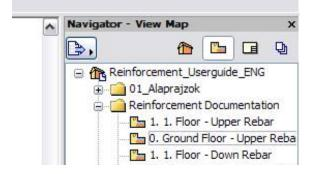
Click "**OK**" button. The view will appear on the navigator under the "**Map View**" tab. We recommend to create a separate folder for the reinforcement plans with the name "**Reinforcement plans**" and then to paste the created views to this library.
