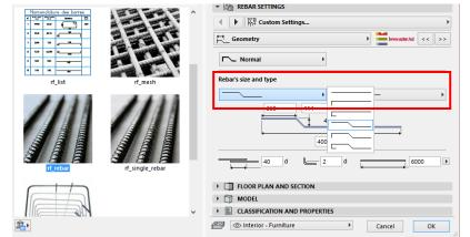
If you need more rebars in the crowning, go back to the Floor Plan view and multiply your rebar object on the Floor Plan to the right positions.
