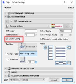
There is a switch in every element "for Listing". Sometimes, some elements are only placed for a complex element's creation in the model space, or maybe an explanation, and irons as outstretched views. In these cases, these irons can be missed out from the optimization and listing. This switch is basically switched on so every element will be listed. When switching off, be careful so that you don't miss out elements what you want to show in the list from the listing.
