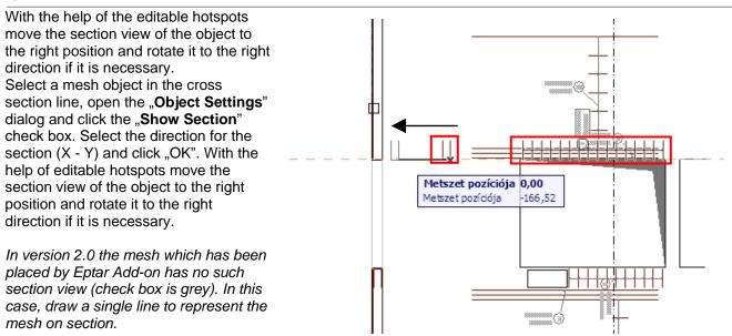
Use the process above to all objects, which is affected in the section view.
