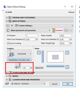
On the Mesh placement and geometry page, you can choose between bottom or top reinforcement. After you choose the bottom or top reinforcement, you can specify the value of concrete cover. This function works only for Horizontal Position. Otherwise, you can only specify concrete cover, which measures concrete cover from the selected side of the wall.
