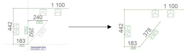
The polygon style rebar can be placed as a single rebar or multiplied for a length.
