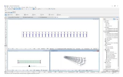
Select the "**rf\_rebar**" object from the library. On the user interface select "**Horizontal**" placement option and click "**Only one rebar**" check box.
