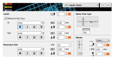
In Reinforcement 3.1 you will find further global setting options. You can define the default settings for the appearance of the views, labels and dimensions of the rebar element.
