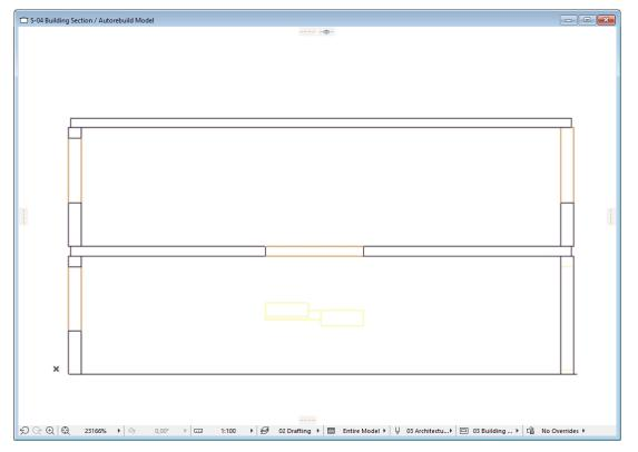
Set up the "**M-1**" Section as a "**Trace**" view in Section "**V-1**". Open the "**M-1**" section view and set up the "**Layer Sets**" to show the slabs in the model in "**Wireframe**" mode. If you do followed the steps, the rebar objects will be visible in the "**M-1**" section.
