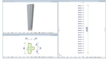
Use the editable hotspots to define the correct height of the stirrup group and change the stirrup's distance if it is necessary (for more information about stirrup placement see point 2.3).
