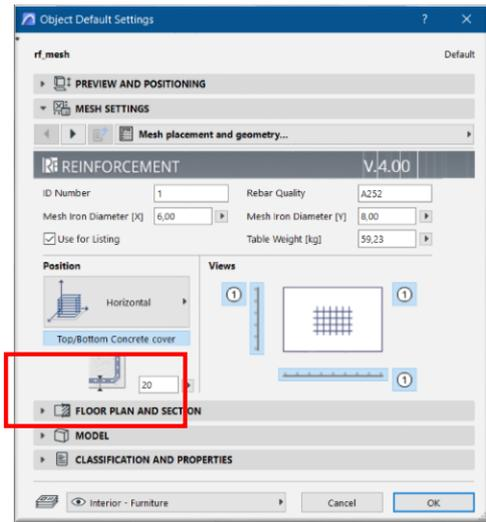
On the Mesh placement and geometry page, you can choose between bottom or top reinforcement. After you choose the bottom or top reinforcement, you can specify the value of concrete cover. This function works only for Horizontal Position. Otherwise, you can only specify concrete cover, which measures concrete cover from the selected side of the wall.
