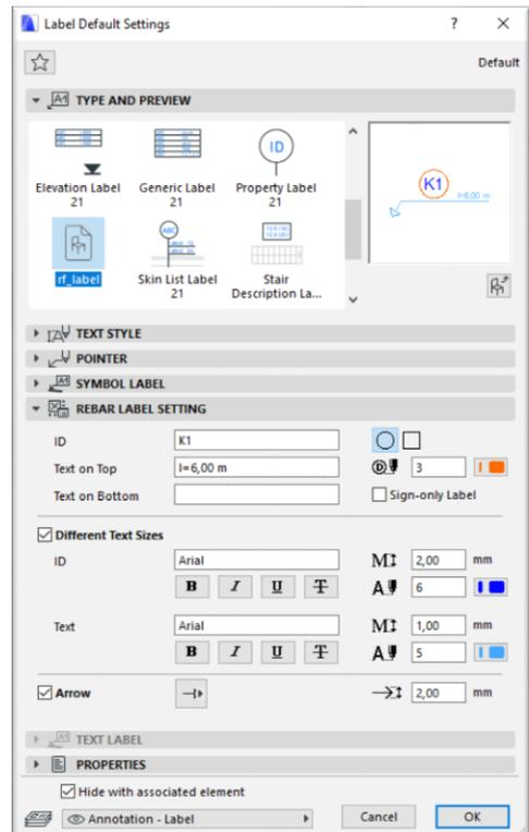
On the working area select the „**Label connection to objects**” placement method. In this case, the settings of the label, such as text and shapes, will be set directly on the Reinforcement object interface, in the Label tab. By choosing the „**Independent**” placement method, the changes are set in the Label Default settings.
