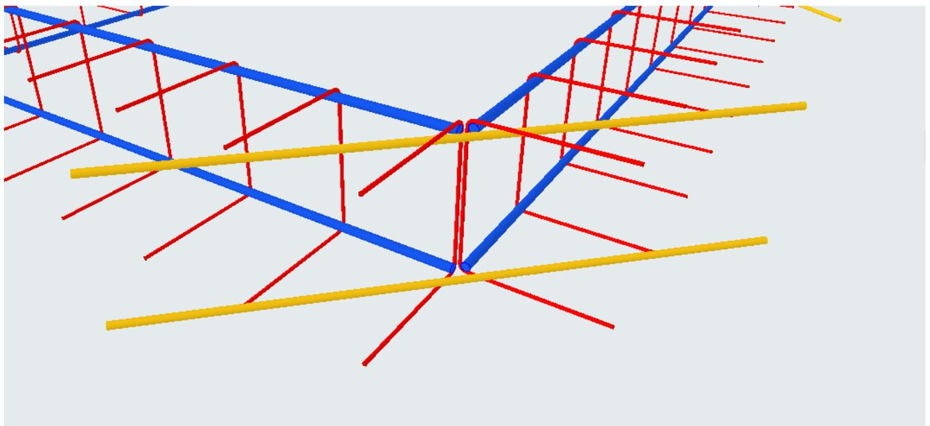
You can modify the parameters of the placed element by selecting it. Select it and open the Object settings window. You can immediately see that there are many more options compared to the settings that appear when you place them. The numbering of the rebars and stirrups can be adjusted per edge.
