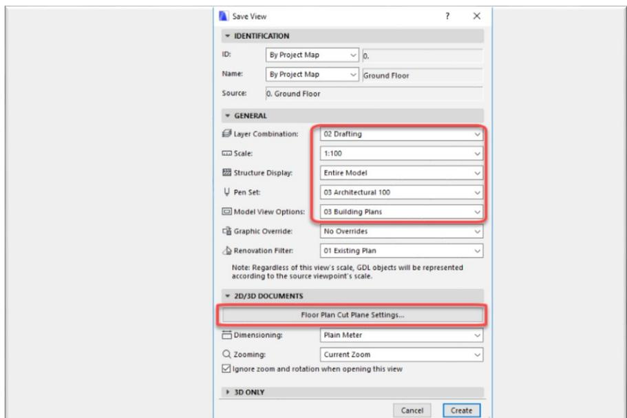
Click the „OK” button. The view will appear on the navigator under the „View Map” tab. We recommend to create a separate folder for the reinforcement plans with the name „Reinforcement plans” and then to paste the created views to this library.
