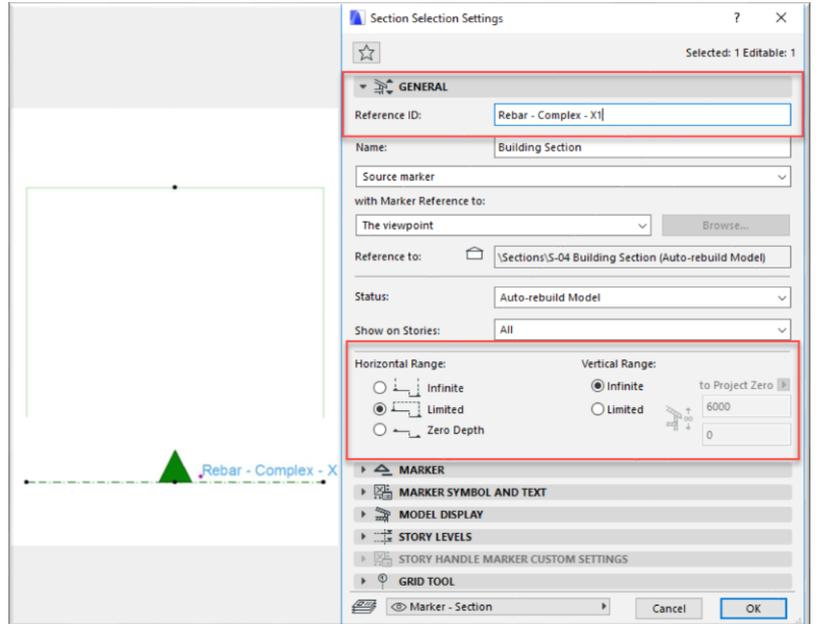
Move the copy of the section on the Floor Plan and rotate it with 90 degrees, these two sections will represent the front and side view. Change the name of the copied section to „**Vas – complex – Y**”.
