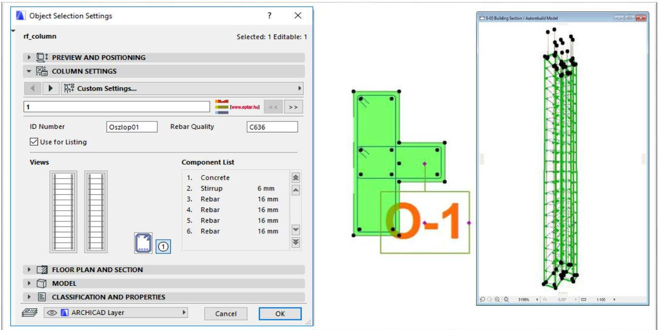
You can check the components of the column objects in the „**Objects Settings**” dialog under the „**General Settings**” tab page but these components are not available to change in this view, you can edit the components only with the help of the command „**Floating palette / Crowning / Edit Crowning**”.
