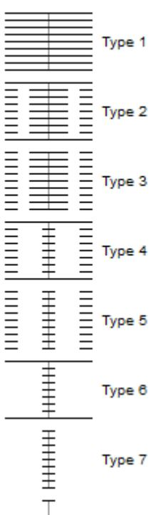
The 2D representation mode and the placement method can be defined with editable hotspots of horizontally placed rebars. Based on the hotspots' position the 2D representation can look different:
