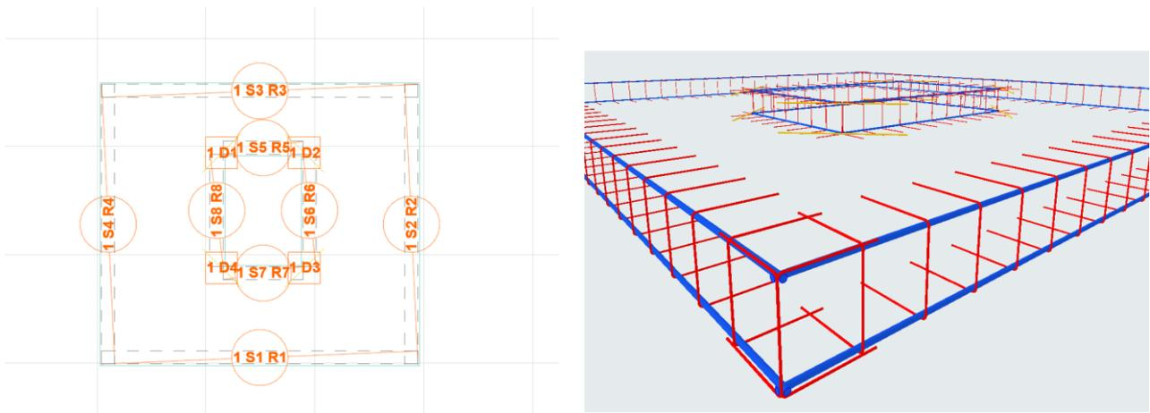
A diagonal iron can also be defined at the corners of the openings, the length of which can be adjusted by adding a value or graphically, it can also be turned off completely.
