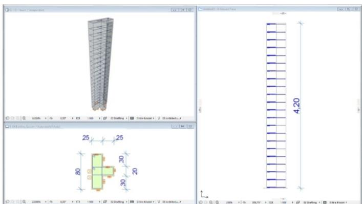
Select the „**rf\_stirrup**” objects from the library. Open the „**Object Settings**” dialog and choose the „**Vertical**” placement option on the „**General**” tab page. Choose a shape for the stirrup and set up the parameters. Click the „**OK**” button and place the stirrup object inside of the „**rf\_concrete**”. Connect the stirrup corners to the hotlines and hotspots which define the safety concrete covers.
