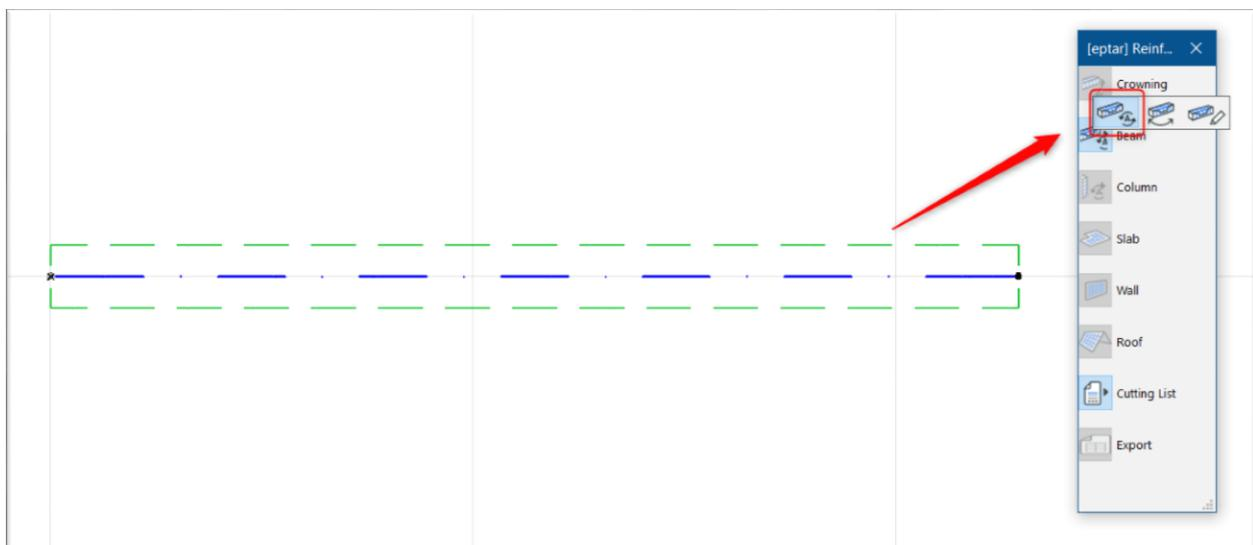
The **rf\_beam** element will be preselected, and you can set all parameters for the current column. These settings are already well known, because the **rf\_beam** element is the same as it was in previous versions. Set all necessary parameters, and click on OK, the add-on will place the correct reinforcement in the column construction.
