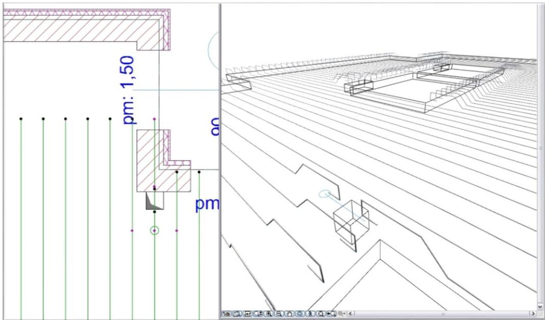
The rebars and meshes - which have been placed with Éptar's add-on - will be grouped together, so the styles of the rebar or meshes will be in one placed group.
