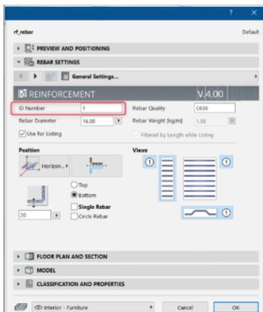
Every element can be given a separate serial number. If you would like to customize the name of the rebars, it is possible. In this case of creation or refreshing of detection of bars, the solution only checks if bars with the same serial numbers have the same properties. If you’ve made a mistake and you’ve given two different bars the same number, the program will renumber one of them.
