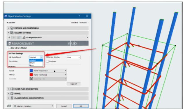
The appearance of the elements in the 3D window can be complex or basic. Complex view gives a chance to see possible overlaps and collisions but can slow the progress/visualization a lot. In basic view, we replace elements with 3D lines so this way the progress/visualization will be much faster and editing will be easier.
