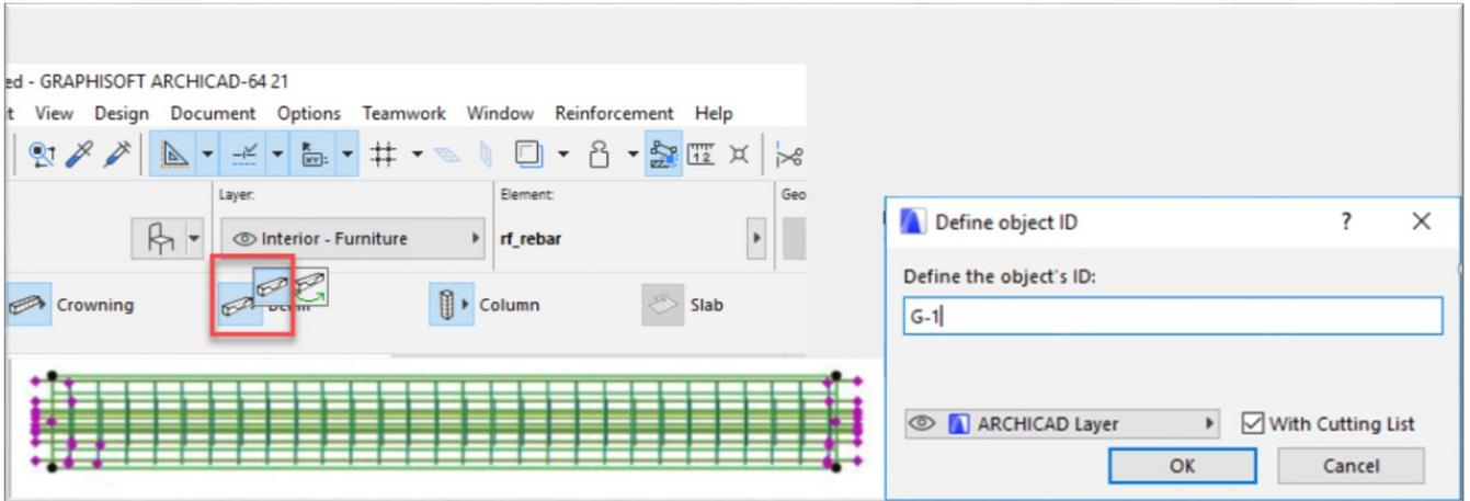
individual rebar table about this construction on the Floor Plan (useful for detail drawings). Click the „OK” button.
