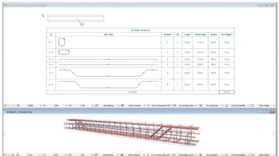
We suggest to copy the cutting list into the detail window. Open the „**Vas – complex – X**” section window and copy the front view from the window to the detail window over the top view. If you need the section view as well, open the „**Vas – complex – Y**” section and copy the side view near to the front view.
