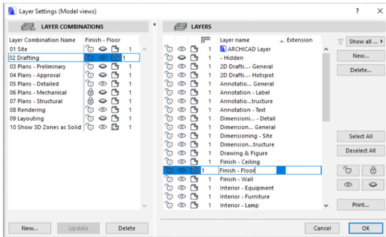
Open „**Document / Layers / Layer Settings**” menu. Among the layers, create (top right button) new layers for the reinforcement plan. We recommend the creation of the following layers:
