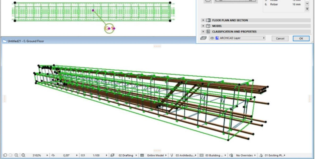
Select the „**Detail Window**” with the name of the column to edit (e.g. G-1). Copy the section view components from the detail window to the Floor Plan.
