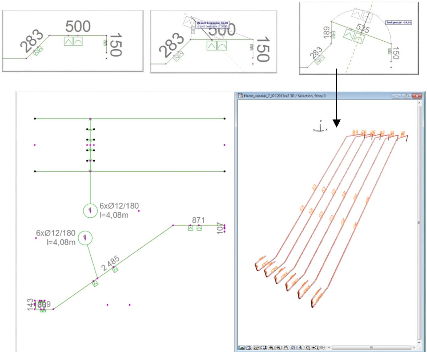
If you want to delete a corner from the polyline move it over the next corner point, the solution will remove the line sections of 0 cm length and the two corner points will be merged.
