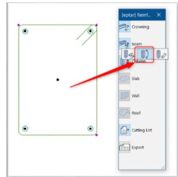
Place the column object on the Floor Plan, at least one copy of it (you can copy this column to multiply it on your plan. It is also suggested to save this object to the „Favorites”). If you requested a cutting list you also can place it into the Floor Plan.
