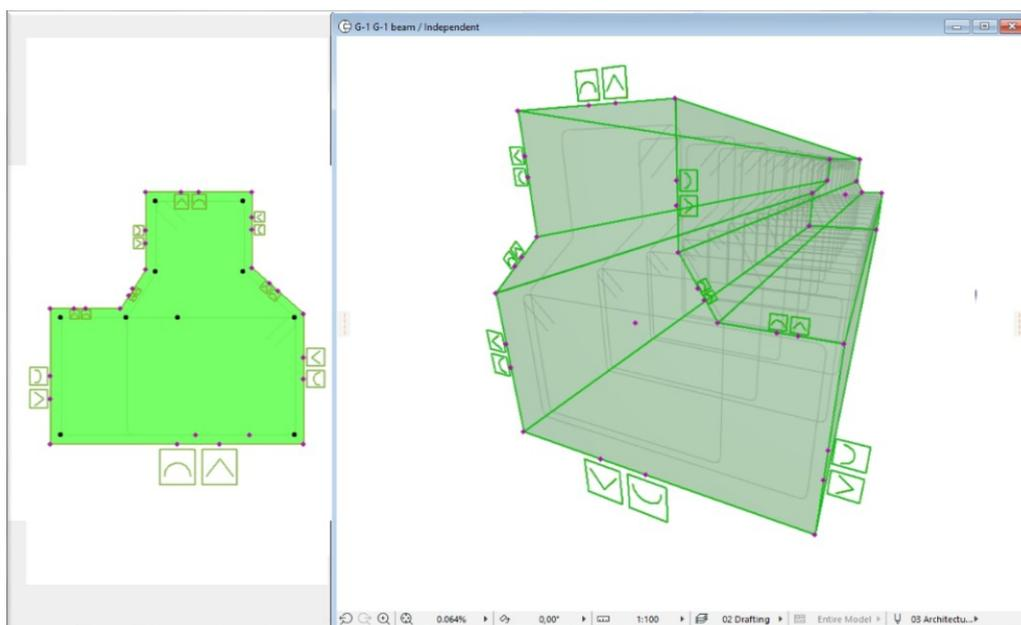
These objects are not available in the cutting list and do not count in the Rebar optimization method.
