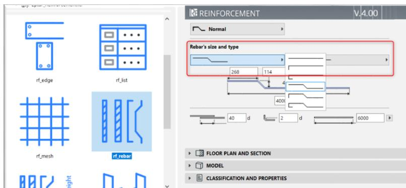
If you need more rebars in the crowning, go back to the Floor Plan view and multiply your rebar object on the Floor Plan to the right positions.
