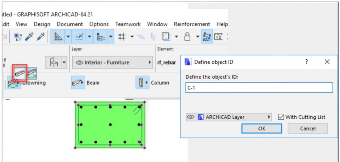
Place the crowning object into the Floor Plan, at least one copy of it (You can copy this crowning to multiply it on your plan. It is also suggested to save this object to the „Favorites”). If you requested a cutting list you also can place it into the Floor Plan.
