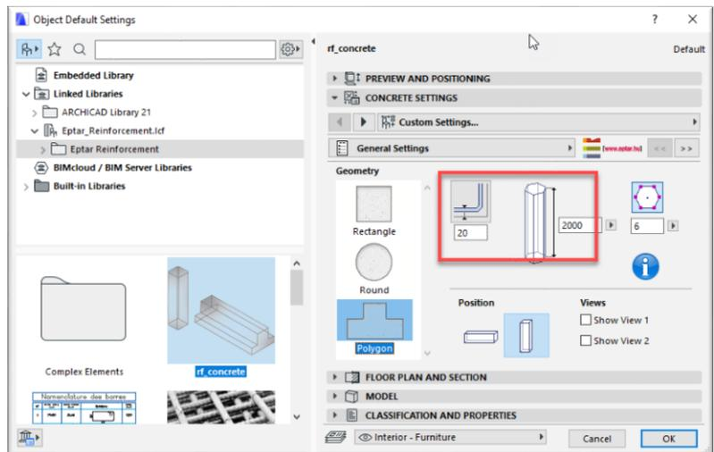
Normally, the columns and beams have a constant section along the full length, so one concrete object is enough to define the external shape of the complex element. If you need more complex shapes, you can use more concrete elements to define the final shape.
