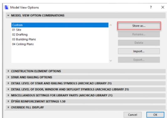
Open „**Document / Set Model View / Model View options**” window. In the appearing dialogue choose „**04 Civil Engineer View**” type. ArchiCAD at this kind of display format only shows the contour of the walls and openings, however, we can set an individual display format too.
