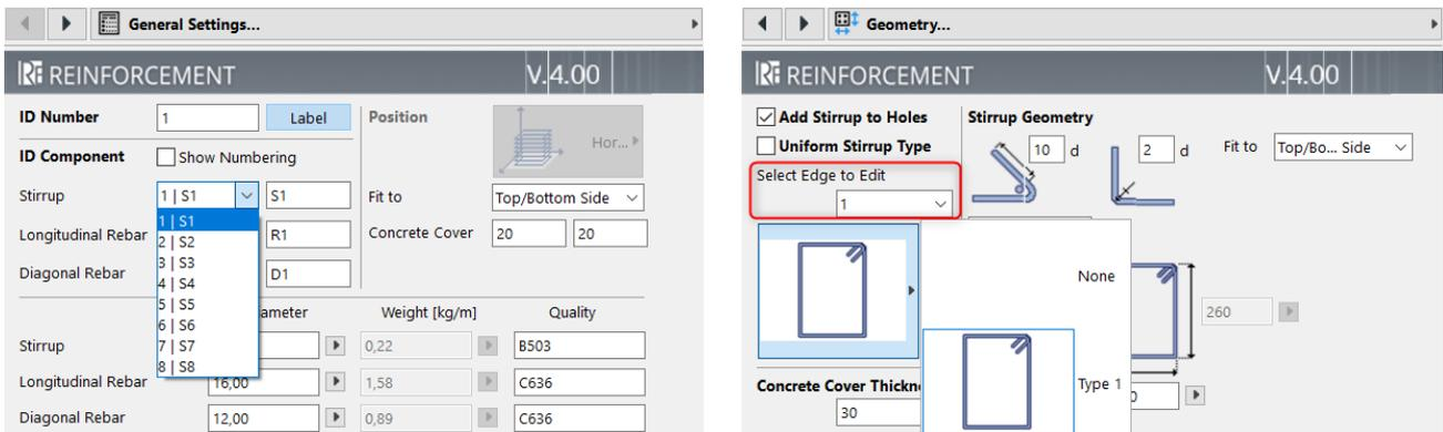
In the next window, you can choose a stirrup type for each edge individually. You can also set the type of stirrups on the floor plan from a graphic menu. If you choose the "no stirrup" option, the reinforcement will not be defined on that edge.
