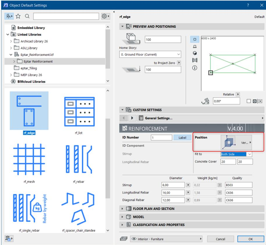
The cursor changes to an "eye" shape, and the rf\_edge element is placed by clicking along the walls.
