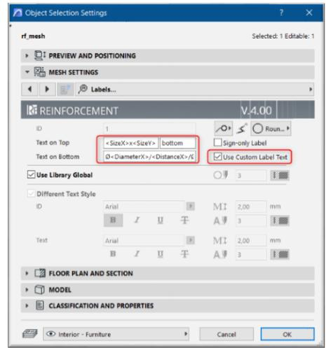
If you would like to use different text on a different views of the placed reinforcement element, go to next 3 pages. Here you can turn on the “Different Main Label”, Different Section Label” or the “Different Side Label” checkboxes, and apply different text contents in the labels.
