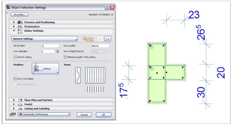
In the opening dialog fill out the name (ID) of the new column (if you choose a name, which already exists, the application will ask you to choose another name). After the definition, you can place this column with this name to the model. The rebar calculation table will contain this name for the components (rebars, stirrups) of this column as well.
