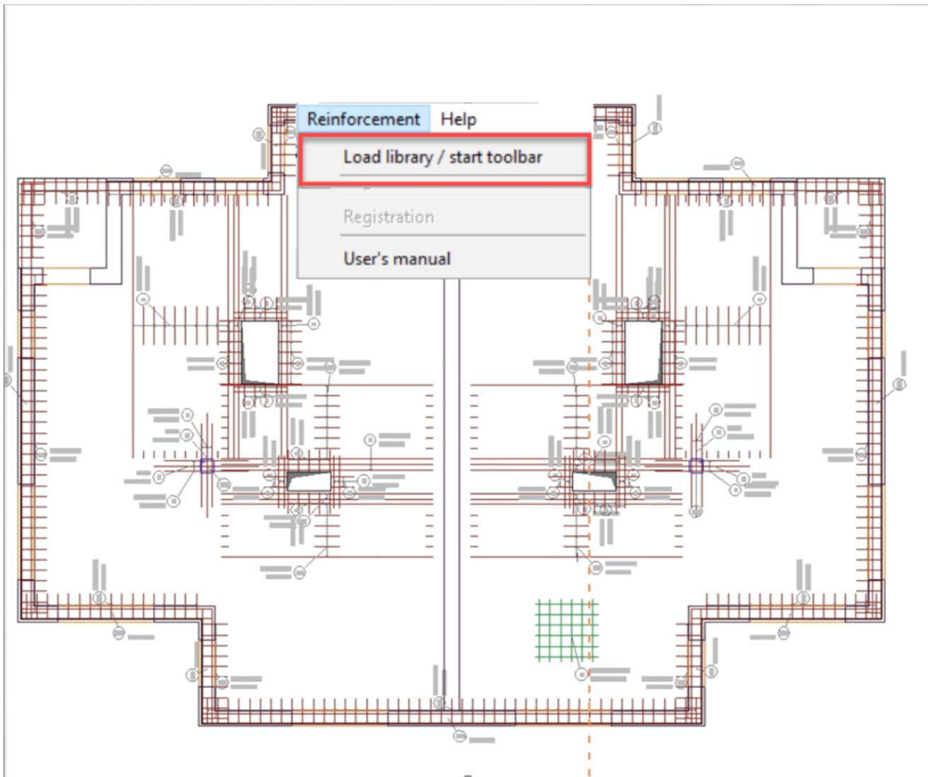
Reinforcement solution helps the users to create the necessary reinforcement drawings and models, it also generates cutting lists and checks the ID mistakes as well.
