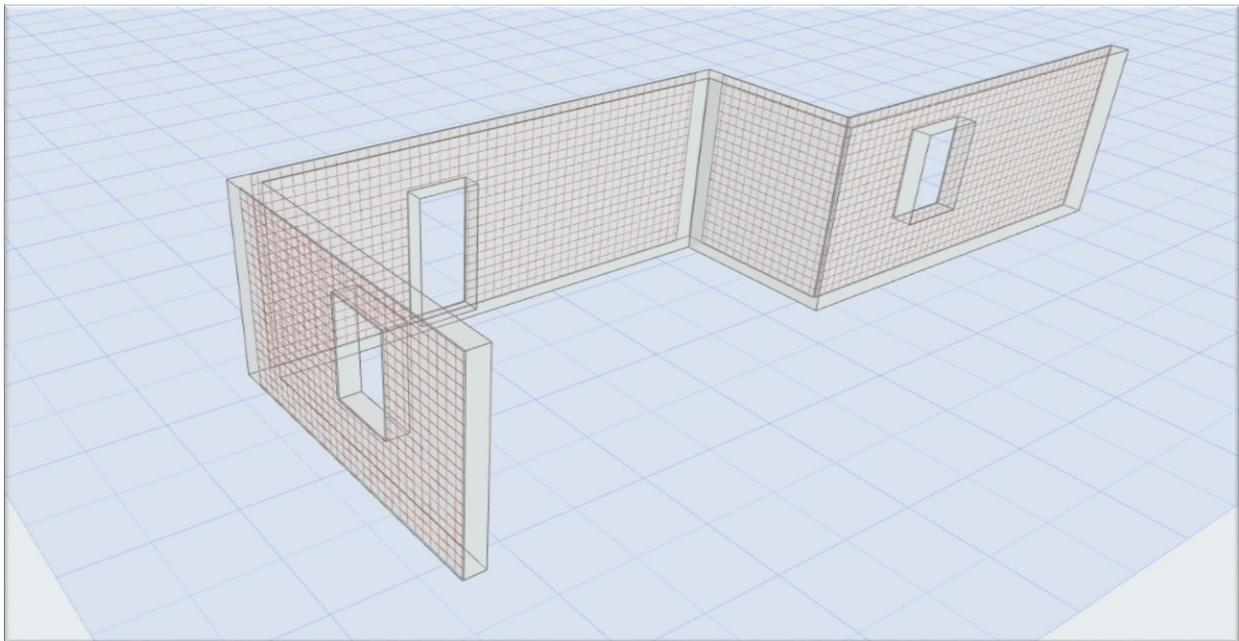
If you define an ArchiCAD slab with holes on the surface the solution can support it, so the rebars and mesh elements do not cross the holes. Please, be circumspect when you define small holes for ArchiCAD slabs (for tubes, mechanical stuffs), because the software does not hesitate to finish a rebar if it crosses the hole and place a new one after the hole. It can cause problems, if you are not careful enough.
