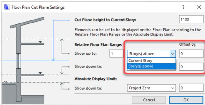
The setting of „Floor Plan Cut Plane Settings” is necessary because that way we can see the upper level’s walls and apertures on layout view.
