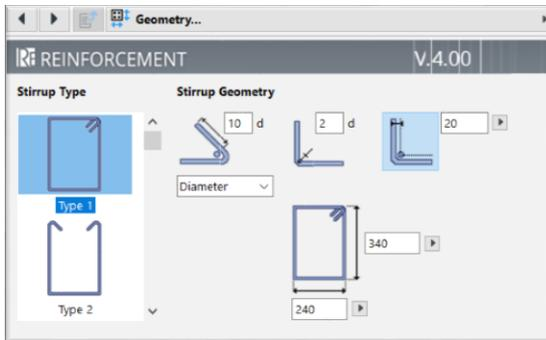
Select the stirrup section form and set up the parameters on the „Geometry” tab page.
