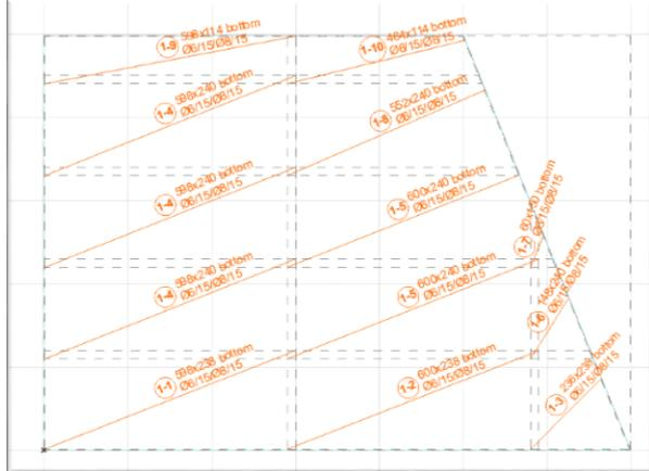
If, due to the shape of the structure, it is simpler or more economical not to distribute the mesh boards at the same time, then its surface can be planned to be laid in several directions. This is a more flexible board layout design because the boards can be rotated according to the shape of the structure, resulting in less cutting loss for cut elements.
