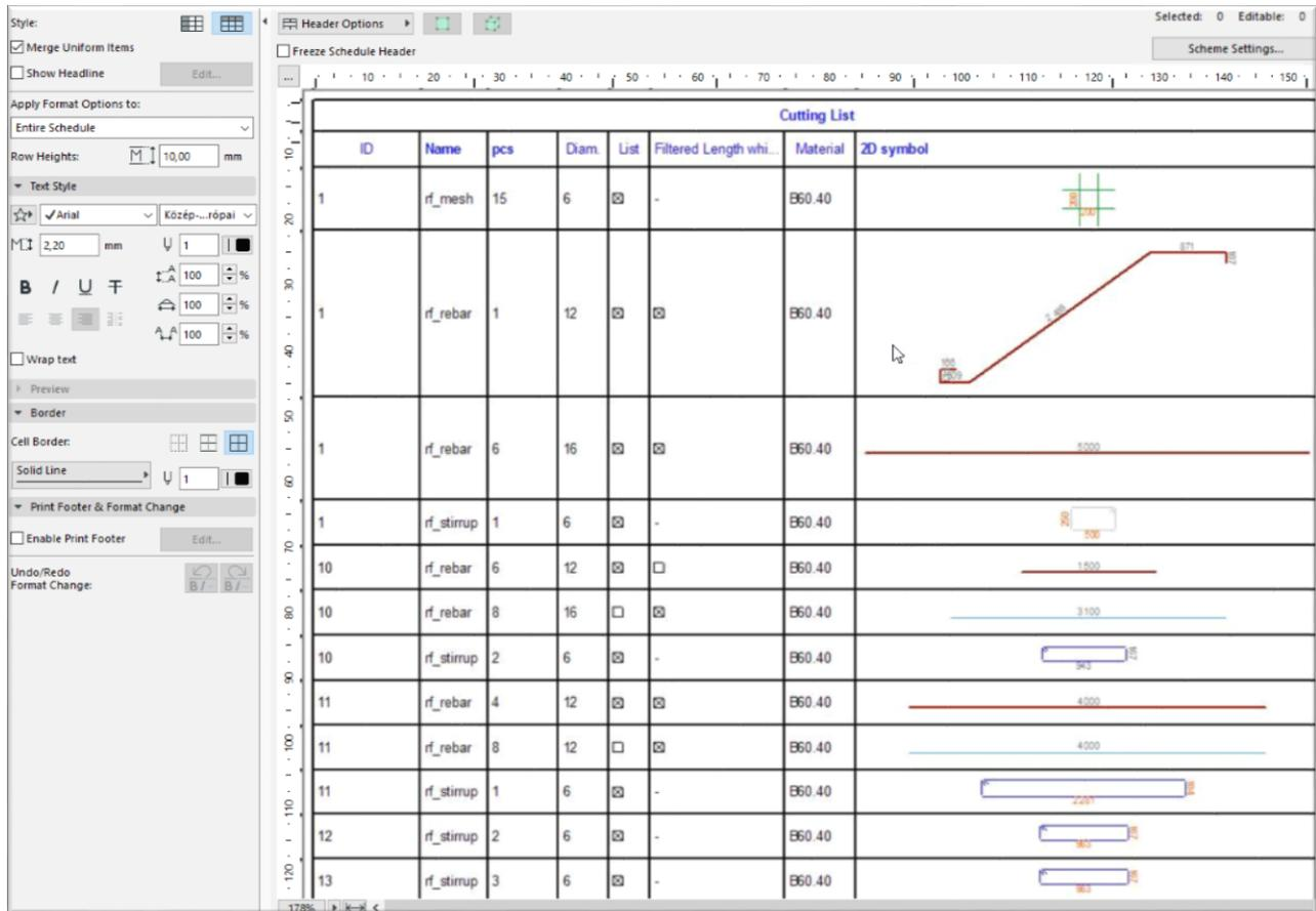
If you can not recognize an object based on the ID or the parameters in the list, you can use one of the buttons on the top of the dialog. Choose one rebar in the list and click the activated button on the header the list. ArchiCAD will show the object on the **Floor Plan** or in the **3D window** immediately.
