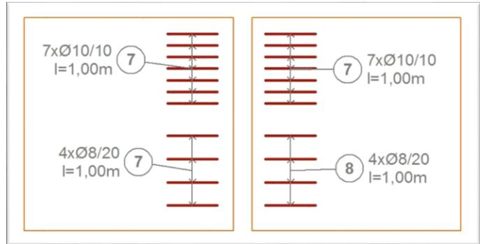
In case you placed objects with different IDs but the parameter values (type, diameter, shape, and length) are the same then the solution will collect them and use them with the same ID. The used ID will be the one which has been placed the most times on the Floor Plan.
