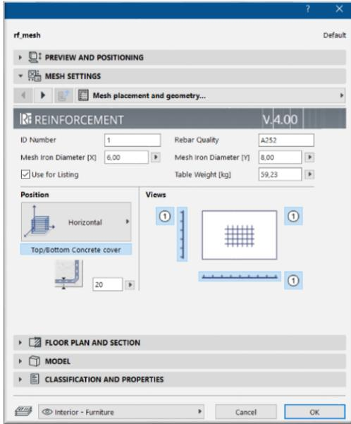
While choosing the mesh object, in the settings window you can set the element’s maximum height in the plan, diameter- holes values (XX x YY), the size of overlapping and the material quality of meshes too.
