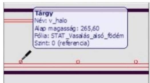
Click on the „View / Zoom / Show all” command. Find the object placed in the last step. Move the object to the right position and rotate it if it is necessary. Set up the label to fit to your requirements.
