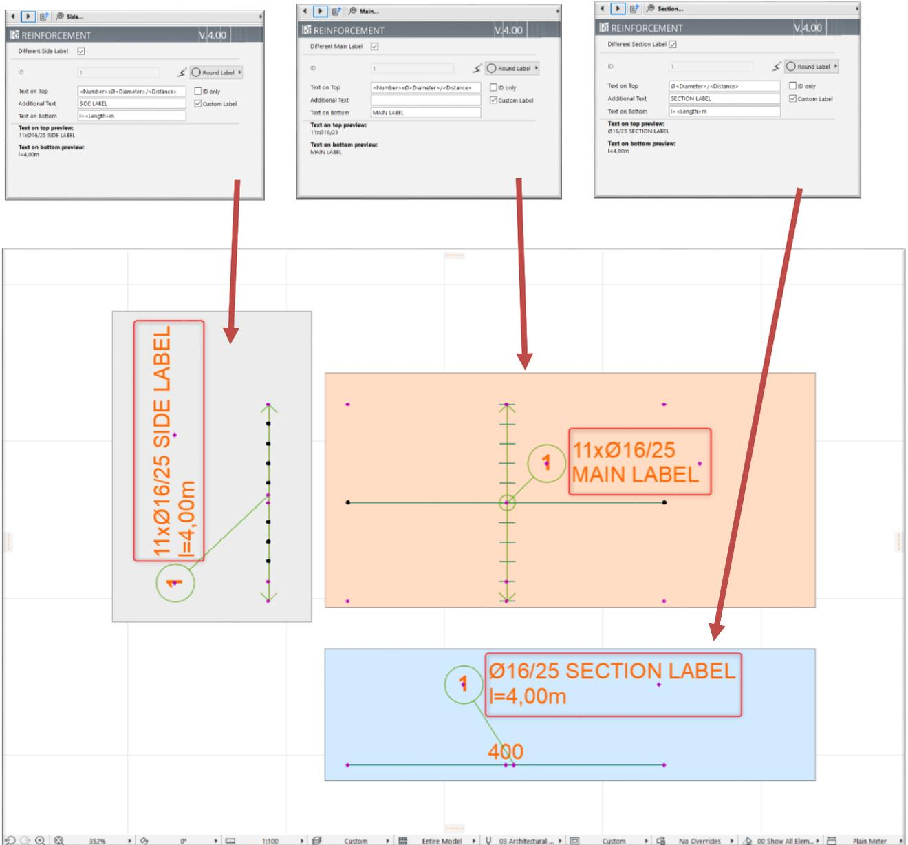
If you want to use the ArchiCAD label option, you can use the „rf\_label” object, what we created directly for Reinforcement solution.
