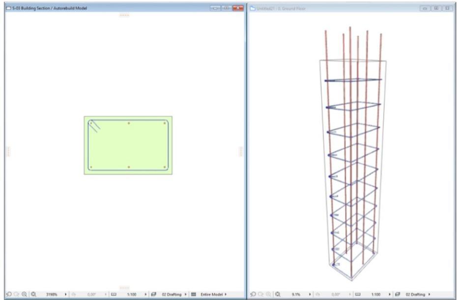
When you are finished with the beam objects rebar structure, select all the rebar, stirrup and concrete elements in the crowning and make sure that the „Use for Listing” parameter is selected.
