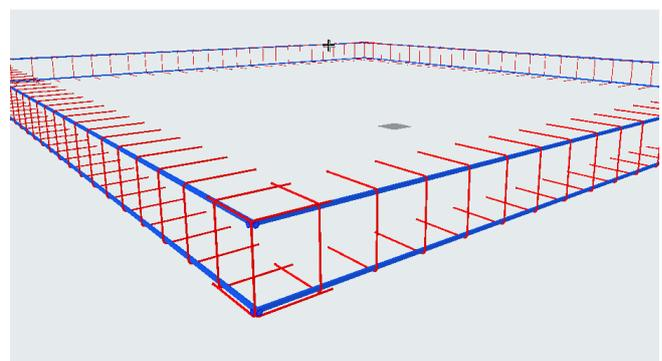
The program also places the reinforcements defined for the outer edges around openings in the slab.
