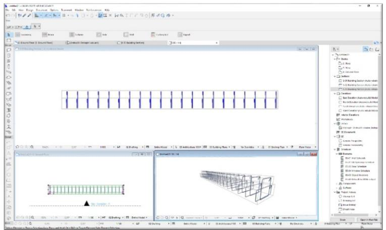
Select the „rf\_rebar” object from the library. On the user interface select the „Horizontal” placement option and click the „Only one rebar” check box.
