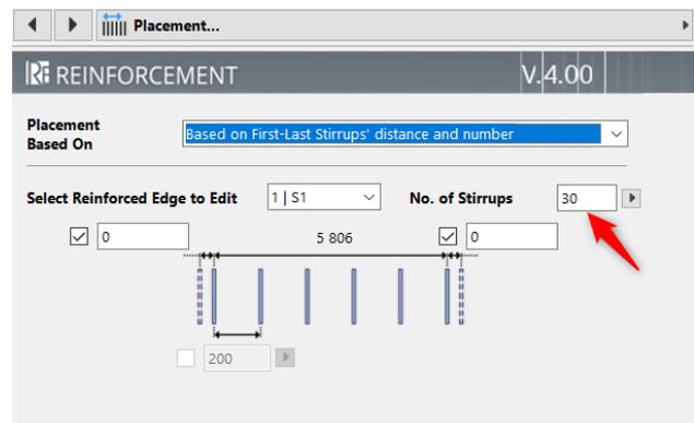
In the next window, you can define the parameters of the rebars per edge:
