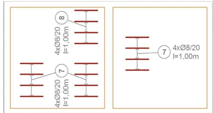
After the automatic calculation and ID check you have to define the position of the cutting list on the Floor Plan. If you have a cutting list on the Floor Plan already, the software does not place a new one but refreshes the existing one.
