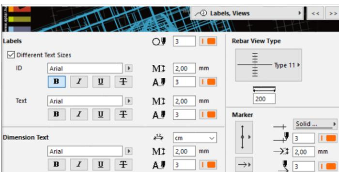
In Reinforcement 4.0 you will find further global setting options. You can define the default settings for the appearance of the views, labels and dimensions of the rebar element.
