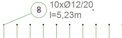
The vertically placed rebar objects' 2D representation is the top view of the rebar. This 2D view
