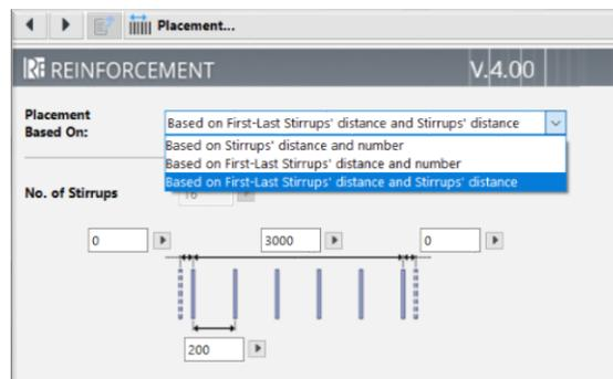
You can edit the distance between the stirrups with editable hotspots on the Floor Plan or in 3D view.
