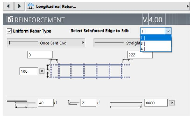
A slanted iron can also be defined at the corners of the openings, the length of which can be adjusted by adding a value or graphically, it can also be turned off completely.
