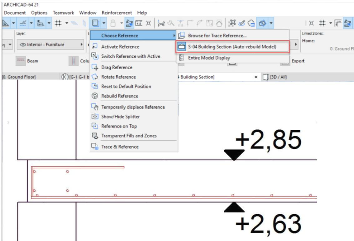
Open the „V-1” section window. In the section view you can see the contour lines of the structures and the 3D section models of the rebar structures (based on the trace drawing). Move your mouse over one of the rebar objects and click on it, while pushing the **Alt + Click**.
