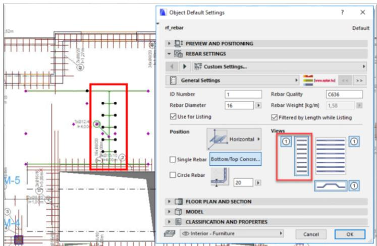
With the help of the editable hotspots move the section view of the object to the right position and rotate it to the right direction if it is necessary. Select a mesh object in the cross section line, open the „Object Settings” dialog and click the „Show Section” check box. Select the direction for the section (X - Y) and click „OK”. With the help of editable hotspots move the section view of the object to the right position and rotate it to the right direction as necessary.
