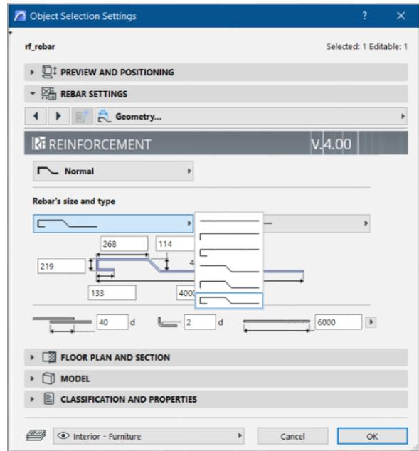
You can choose two options during the rebar’s geometrical definition. The solution can calculate with the full length of rebars but you can ignore this filter and filtering the rebars regarding their end’s structure. If you switch the „Calculate with length” check box during the listing process rebars will be filtered regarding the full lengths, even if they have the same type of endings or not.
