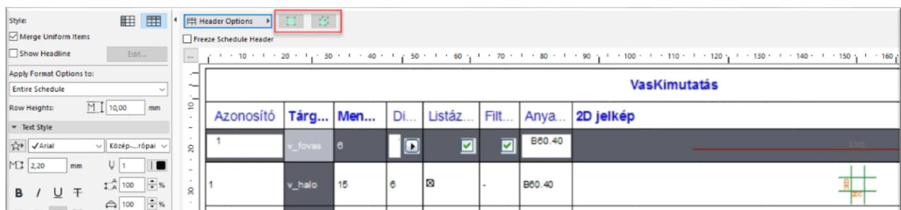
In this schedule you have the possibility to change some parameters of the selected object(s). Select one object in the list and change the diameter or the quality values. These changes will be automatically activated for all placed objects in the model, so you can easily change the IDs or other parameters of the objects.
