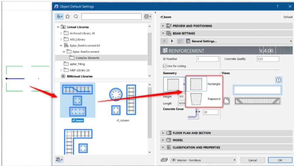
First the beam should be selected. When the beam object is selected, click on the “beam” icon in the Reinforcement palette. In previous versions the first “beam” icon was used to create complex elements, but now the settings window appears.
