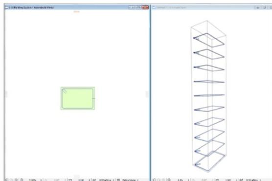
Select the „rf\_rebar” object from the library. On the User Interface select the „Vertical” placement option and switch on the „Only one rebar” check box. Set up the „Straight” style of the endings in the „Geometry” tab page. Click the „OK” button. Place the rebar object inside the stirrup contour. Click on the Section window and move the rebar on the right position with the right length.
