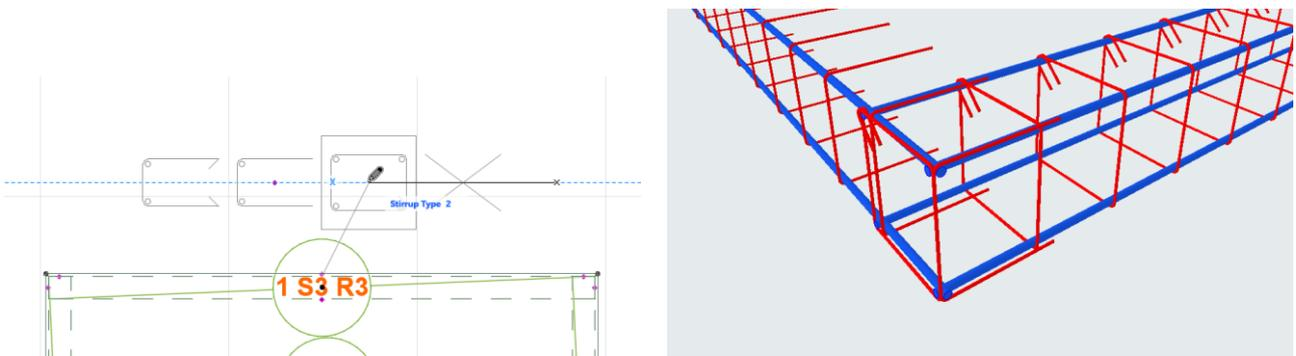
In the case of a closed stirrup, the program automatically defines 4 rebars.
