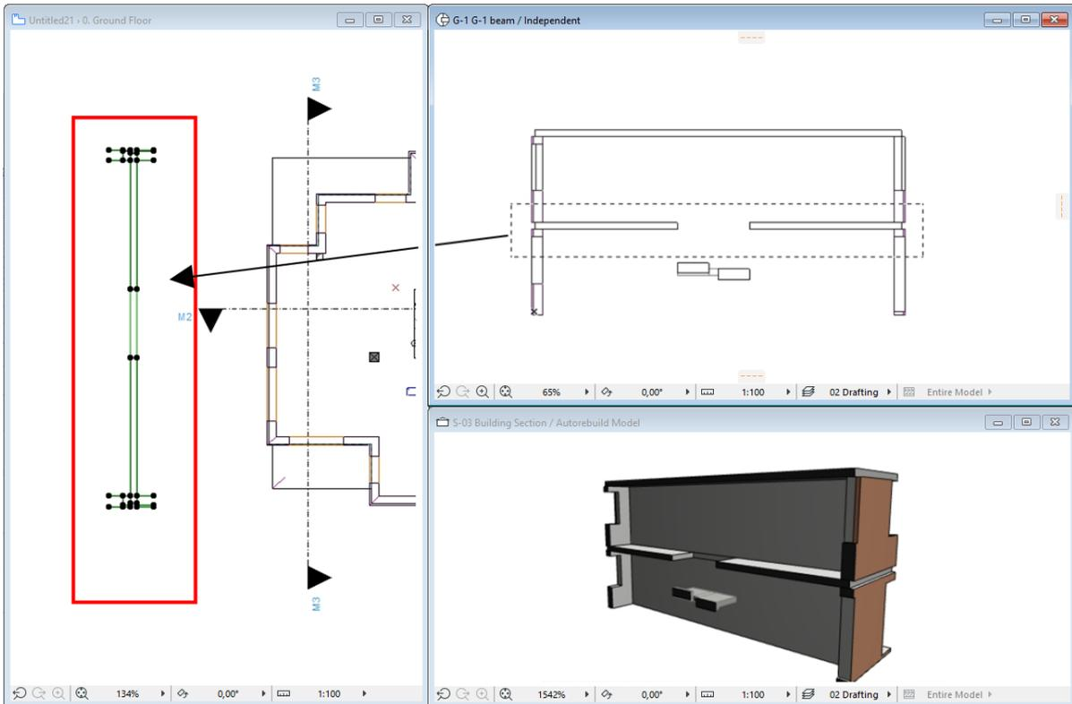
Select one of the rebar objects which cross the section line on the Floor Plan. Open the „**Object Settings**” dialog and click the side view icon on the „**General Settings**” tab page.
