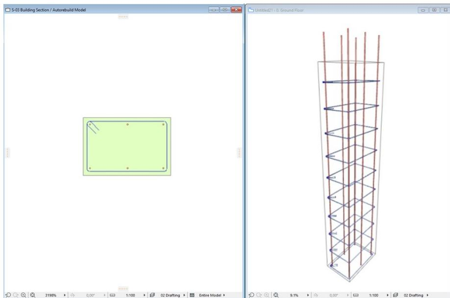
When you are finished with the beam objects rebar structure, select all the rebar, stirrup, concrete elements in the crowning and make sure that the „Use for Listing” parameter is selected.
