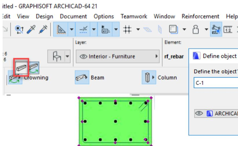
If you click this check box (default), you can place an individual rebar table about this construction on the Floor Plan (useful for detail drawings). Click „OK” button.
