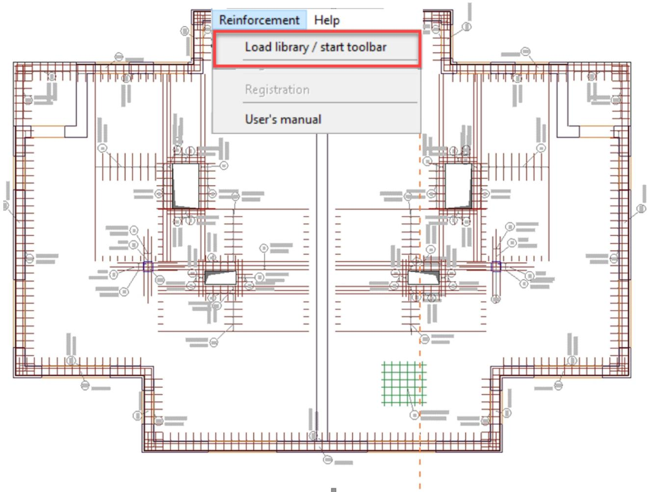
Reinforcement solution helps the users to create the necessary reinforcement drawings and models, it also generates cutting lists and checks the ID mistakes as well. In point 2.5 (complex structures) we have already written about the cutting list definition which is available to be placed on the Floor Plan. You can place the same cutting list for several construction drawings as well.
