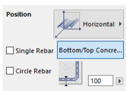
In the placement process you can select to use rebar in horizontal or vertical position. The vertical option helps you to use the rebars to define columns or other vertical style complex elements.
