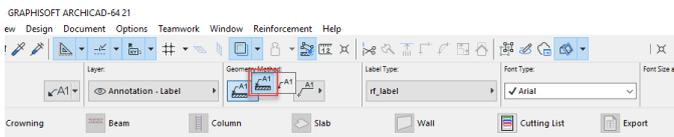
On the working area select the „**Label connection to objects**” placement method. In this case, the settings of the label, such as text and shapes, will be set directly on the Reinforcement object interface, in the Label tab. By choosing the „**Independent**” placement method, the changes are setting in the Label Default settings.
