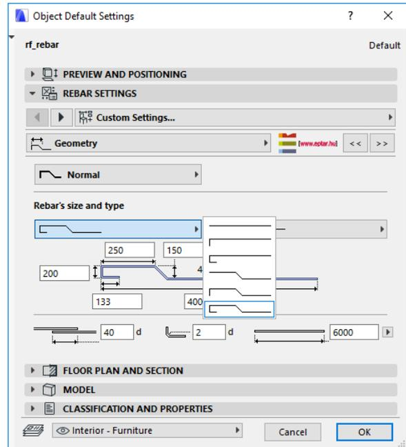
You can choose two options during the rebar’s geometrical definition. The solution can calculate with the full length of rebars but you can ignore this filter and filtering the rebars regarding their end’s structure. If you switch the „Calculate with length” check box during the listing process rebars we will filtered regarding the full lengths, even they have the same type of endings or not.
