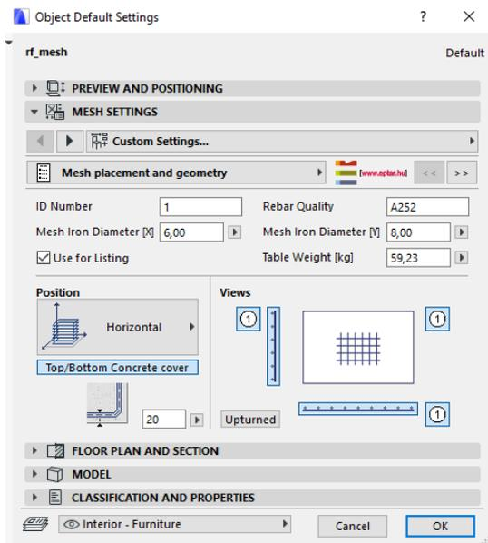
While choosing the mesh object, in the settings window you can set the element's maximum height in the plan, diameter-, holes values (XX x YY), the size of overlapping and the material quality of meshes too.
