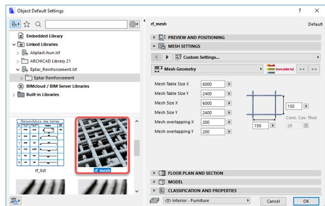
To change the placement direction of the rebar / mesh objects, select the object and click „**Enable polygon editing**” or „**Show Sections**” check box on the Object settings dialog. Click „OK” button. On the Floor Plan you can see the editable hotspots which helps you to define the placement direction and the placement origin.
