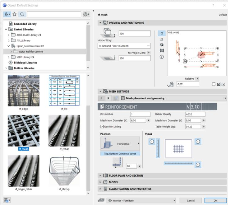
In the dialog (under the „**Geometry**” tab) you can set up the style of the end of rebar and the length of the different parts.
