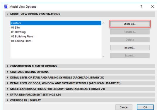
Under the „**Override Fill Display**” tab switch „**Override Zone Fills**”, and „**Hide Zone Stamps**” switches. As it can be seen on the upper side of the dialogue under the „**Set Model View**”, „**Custom**” has been chosen because of the changes made. Click „**Store As**” button and give name „**05 Reinforcement plan**” to the changes. Click OK and close the window.
