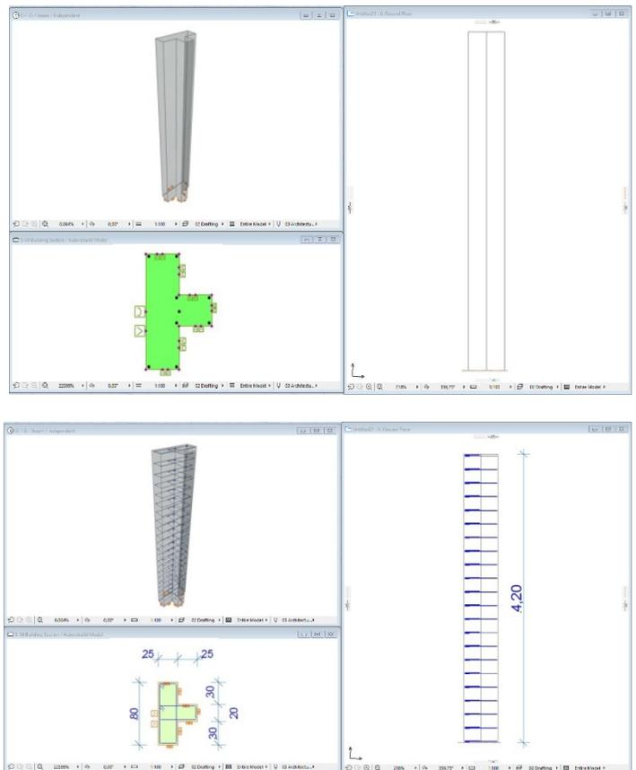
Use the editable hotspots to define the correct height of the stirrup group and change the stirrup's distance if it is necessary (for more information about stirrup placement see point 2.3).
