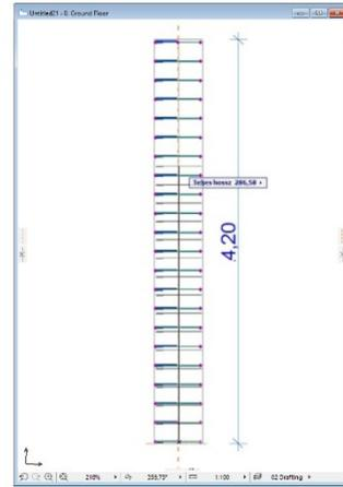
Select the „rf\_rebar” object from the library. Select „Vertical” placement option on the user interface and click „Only one rebar” check box.
