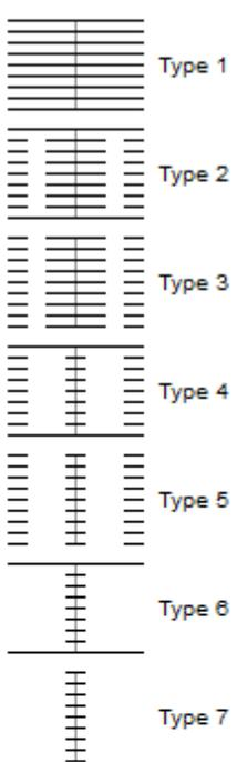
The 2D representation mode and the placement method can be defined with editable hotspots of horizontally placed rebars. Based on the hotspots position the 2D representation can look differently:
