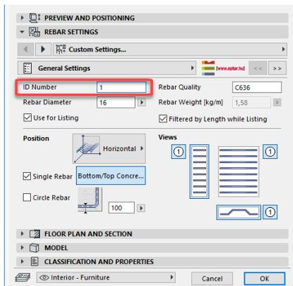
Every element can be granted with a separate serial number. If you would like to custom name the rebars, it is possible. In this case of creation or refreshing of detection of iron, the solution only checks if irons with the same serial numbers, have the same properties. If you’ve made a mistake and you’ve given two different irons the same number, the program will renumber one of them.
