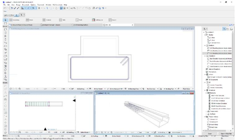
Use the editable hotspots to define the correct length of the stirrup group and change the stirrup’s distance, if it is necessary (for more information about stirrup placement see point 2.3).
