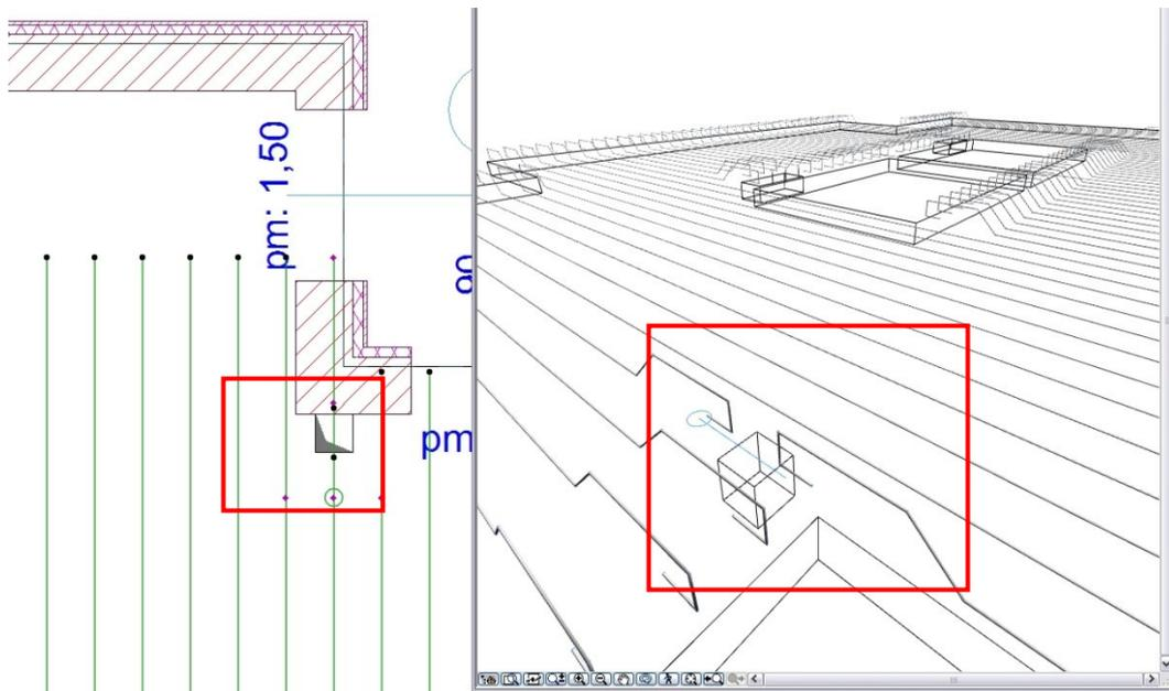
The rebars and meshes - which have been placed with Eptar Add-on – will be grouped together, so the styles of the rebar or meshes will be in one placed group.
