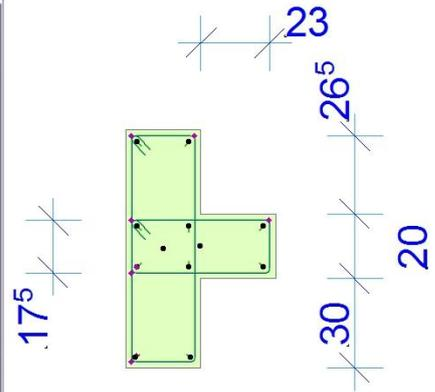
Select all the rebars, stirrups and concrete elements in your construction on the Floor Plan (section view is not supported for this command) and choose „Floating palette / Column / Create Column” command.
