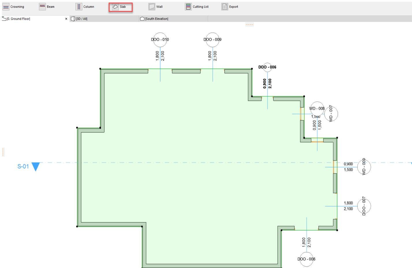
Select the ArchiCAD slab or wall objects to fill out with rebar or mesh elements. Use „**Floating palette / Slab or Wall**” command. Select the rebar or mesh object in the dialog box and set up the necessary parameters as we defined in the earlier chapter. Click „OK” button, the ArchiCAD automatically places the rebar or mesh elements into the polygon shape slab or wall with the parameters already defined.
