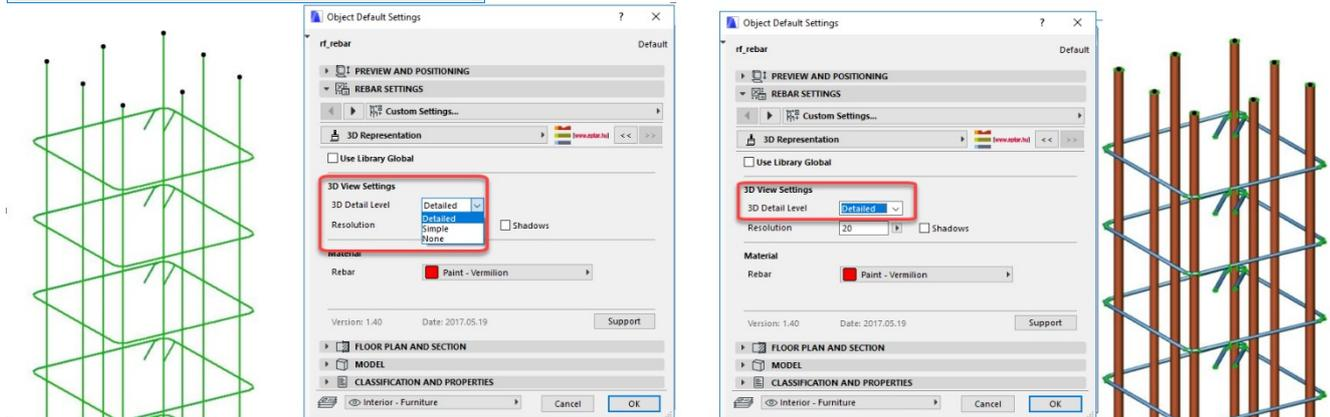
The appearance of the elements in the 3D window can be complex or basic. Complex view gives a chance to see possible overlaps and collisions but can slow the progress/visualization a lot. In basic view, we replace elements with 3D lines so this way the progress/visualization will be much faster and editing will be easier.
