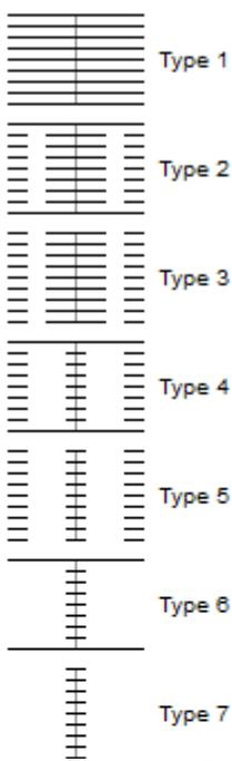
The 2D representation mode and the placement method can be defined with editable hotspots of horizontally placed rebars. Based on the hotspots position the 2D representation can look differently:
