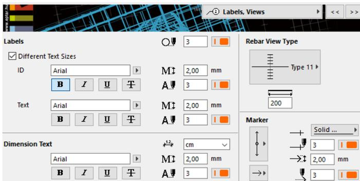
In Reinforcement 3.1 you will find further global setting options. You can define the default settings for the appearance of the views, labels and dimensions of the rebar element.
