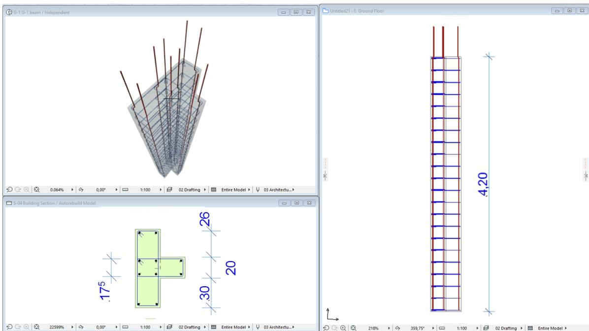
When you are ready with the column objects rebar structure, select all the rebar, stirrup, and concrete elements in the Column and make sure, the „Use for Listing” parameter is selected.
