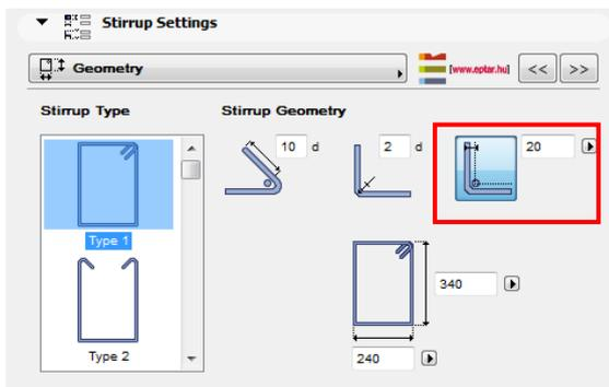
Select stirrup section form and set up the parameters on the „**Geometry**” tab page.
