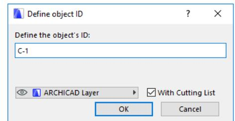
Place the column object on the Floor Plan, at least one copy of it (you can copy this column to multiply it on your plan. It is also suggested to save this object to the „Favorites”). If you requested a cutting list you also can place it into the Floor Plan.
