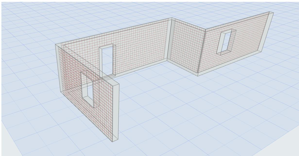
If you define an ArchiCAD slab with holes on the surface the solution can support it, so the rebars and mesh elements do not cross the holes. Please, be circumspect when you define small holes for ArchiCAD slabs (for tubes, mechanical stuffs), because the software do not hesitate to finish a rebar if it cross the hole and place a new one after the hole. It can cause problems, if you are not careful enough.
