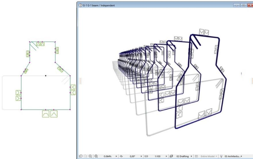
When you finish the shape definition, switch off the „**Editable hotspots**” check box. The small icons will disappear on the 2D view and 3D model.
