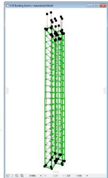
You can check the components of the column objects in the „**Objects Settings**” dialog under the „**General Settings**” tab page but these components are not available to change in this view, you can edit the components only with the help of the command „**Floating palette / Crowning / Edit Crowning**”.
