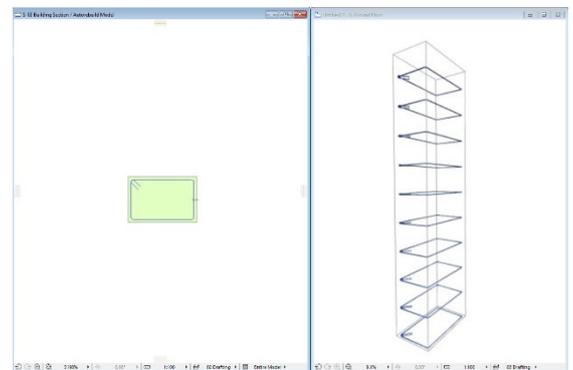
Select the „**rf\_rebar**” object from the library. On the User Interface select the „**Vertical**” placement option and switch on the „**Only one rebar**” check box. Set up the „**Straight**” style of the endings in the „**Geometry**” tab page. Click the „**OK**” button. Place the rebar object inside the stirrup contour. Click on the Section window and move the rebar on the right position with the right length.
