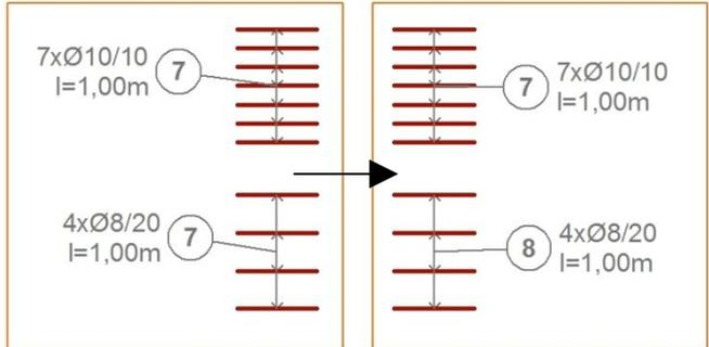
In case you placed objects with different IDs but the parameter values (type, diameter, shape, and length) are the same then solution will collect them and use them with the same ID. The used ID will be the one which ID has been placed more times on the Floor Plan.
