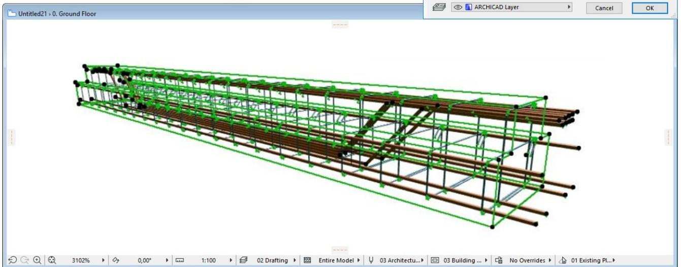
Select the „**Detail Window**” with the name of the column to edit (e.g. G-1). Copy the section view components from the detail window to the Floor Plan.
