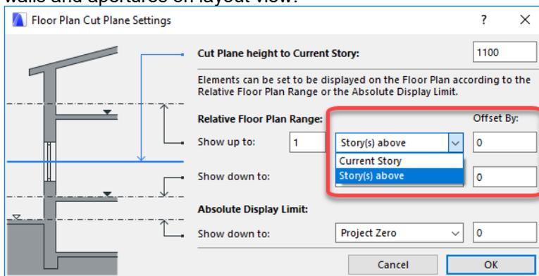
Click „Floor Plan Cut Plane Settings” button. In the appearing dialogue next to the „Show Up to” switch, switch the value from 0 to 0.5 meter and „Show Down to” switch to „Current Story” 0.5.
