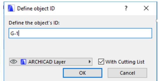
this name as well for the components (rebars and stirrups) of this column. In the dialog, you can see a check box with a name „With List”. If click this check box (default), you can place an individual rebar table about this construction on the Floor Plan (useful for detail drawings). Click „OK” button.
