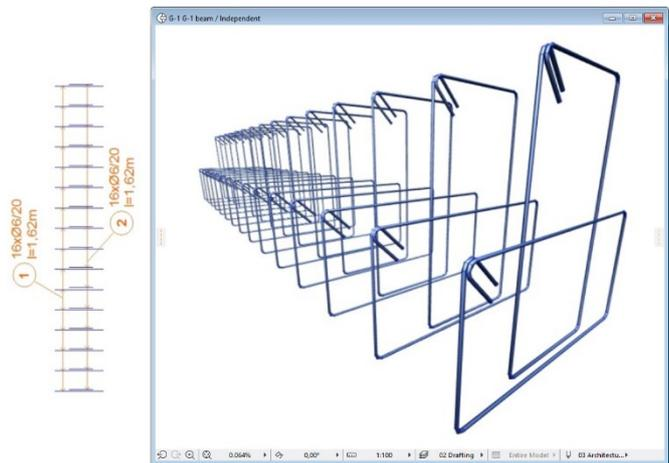
On the Floor Plan, you can switch on the Label for the object on the „**2D Representation**” tab page. You also can use the original ArchiCAD label elements, find more details about this functionality in point 2.8.
