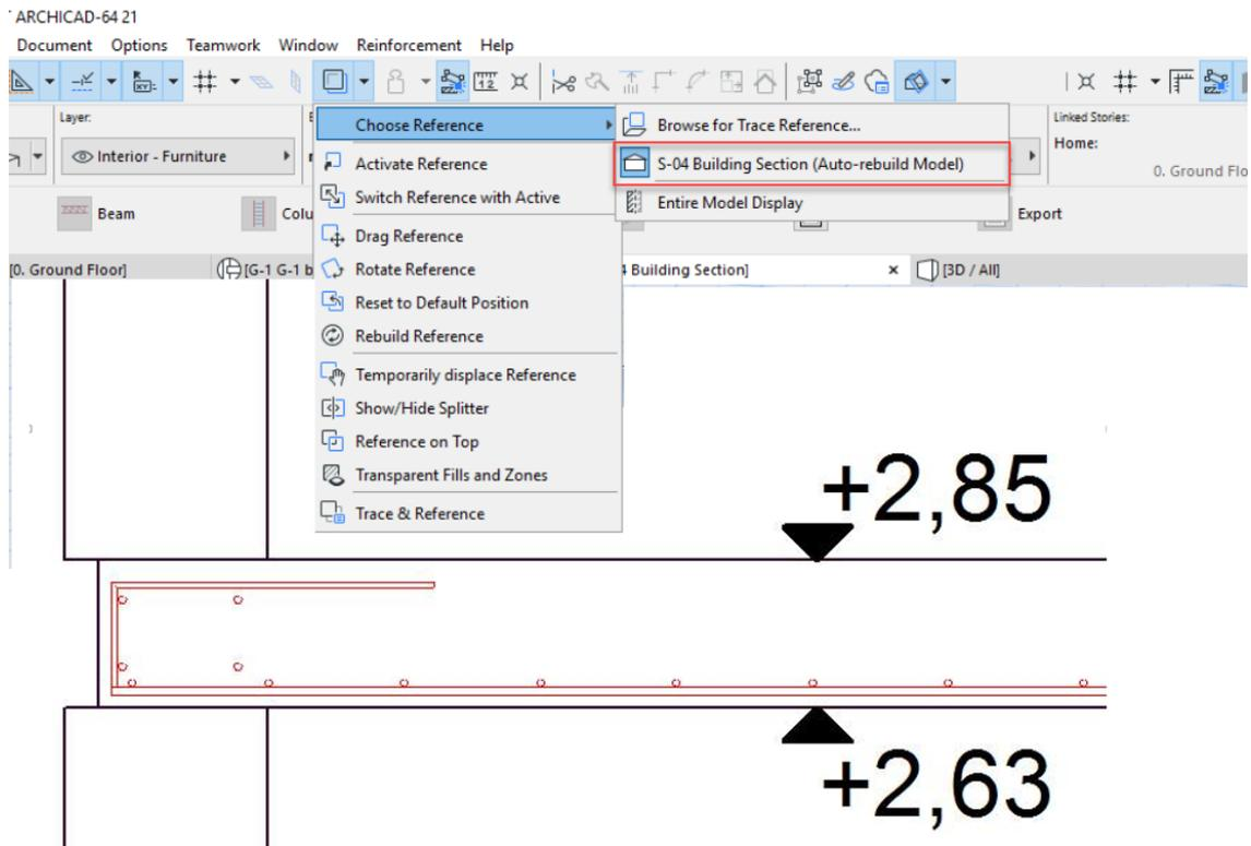
Open the „V-1” section window. In section view you can see the contour lines of the structures and the 3D section models of the rebar structures (based on the trace drawing). Move your mouse over one of the rebar object and click on it, when you push the **Alt** button (**Alt + Click**).
