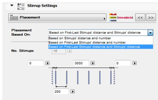
You can edit the distance between the stirrups with editable hotspots on the Floor Plan or in 3D view.
