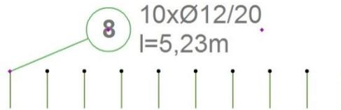
The vertically placed rebar objects' 2D representation is the top view of the rebar. This 2D view is not able to
