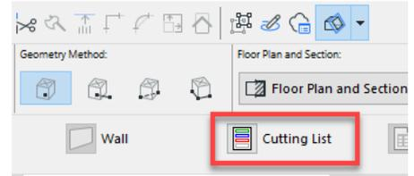
In case you placed objects with the same ID but the parameter values (type, diameter, shape, and length) are different then the solution will change the ID number of one of them.
