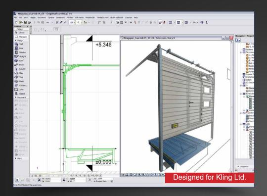
The ArchiCAD library contains the full product range of gate manufacturer. The GDL library has a simple configurator interface to set up all the necessary parameters for design and manufacturing. The library is available in English language as well.
