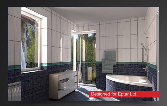
ArchiCAD solution for room tiling. User can define tiles, sizes and listing parameters. 2D drawings and 3D model definition in one, easy step.
