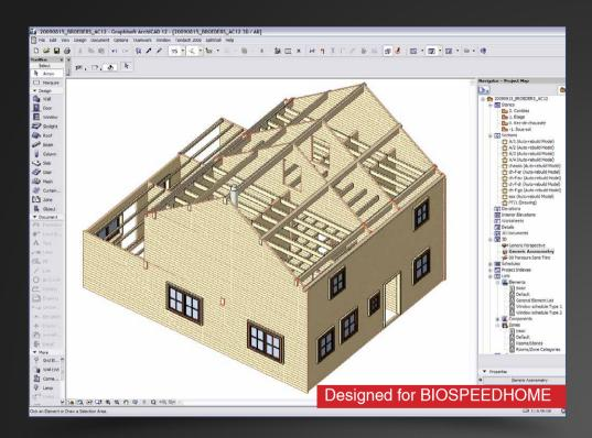
Our client wanted to control the CNC cutting machine directly from ArchiCAD. We developed an application to define log cuts and drills in ArchiCAD. The final result is a tabtext file, which can be used by the CNC machine directly.
