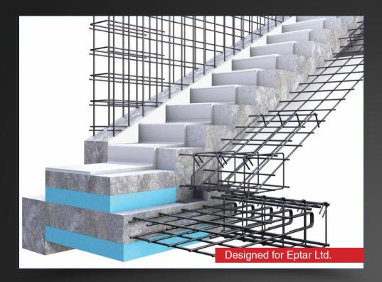
This library was developed to support Civil engineers, who want to work with ArchiCAD. The application helps to model the reinforcement bars in 2D and 3D as well. After the rebar placement, users can simply collect rebar items, optimise the ID numbers and create cutting lists.
